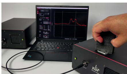
Sample 1. Reflection measurements of a black foam.
