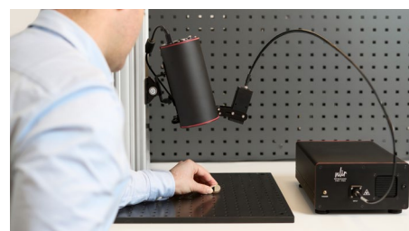
Performing reflection measurements using NLIR's MIDWAVE Spectrometer and REFLECTION Interface.
