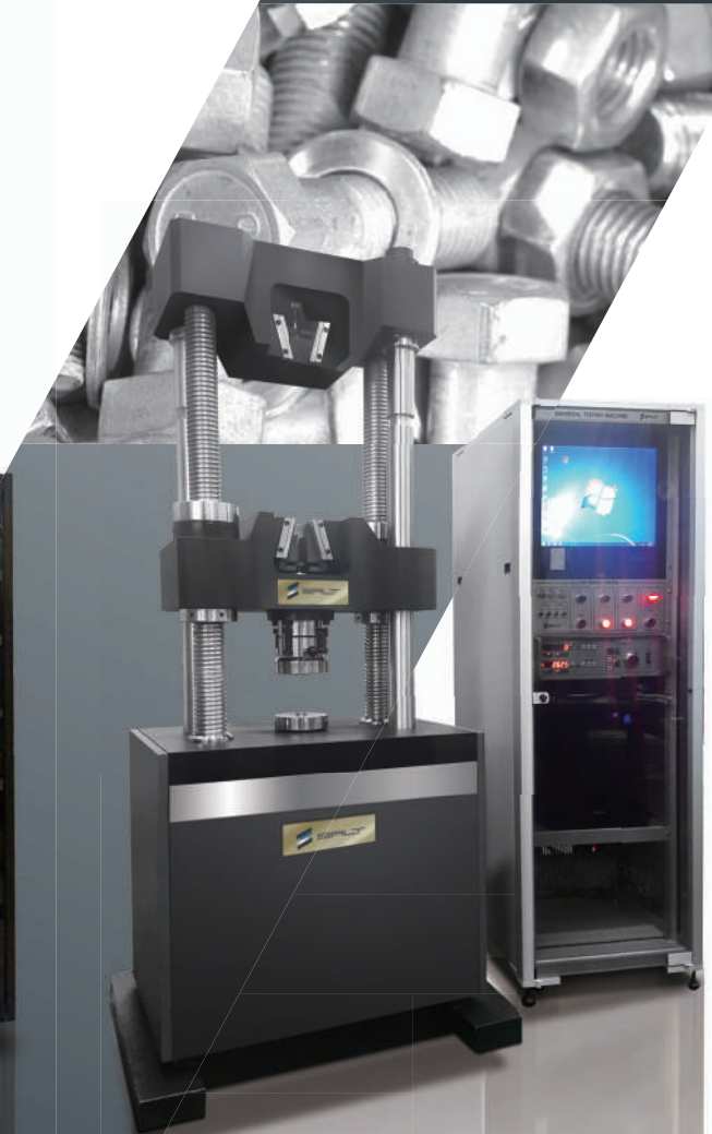
ST-1004 4 Column Structure Type
