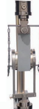
Drum Peel Jig ASTM D1781
